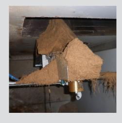
Pneumatic compaction unit for wood chips and sawdust
